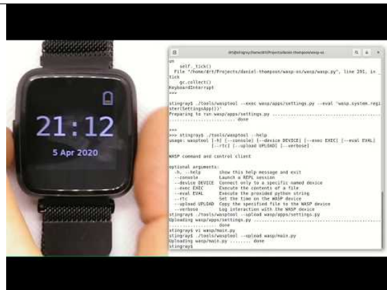
Fig. 4: How to develop wasp-os python applications on a Pine64 PineTime
