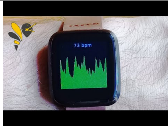
Fig. 2: Open source heart rate monitoring for Pine64 PineTime
