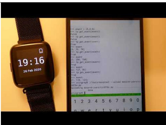
Fig. 5: Developing for Pine64 PineTime using wasp-os and MicroPython
